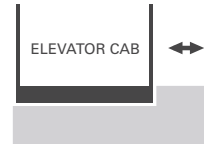
Slab with RAM's 2in Pit
