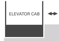
Typical Competitor 6-12 in Pit (requires extensive ground prep)
